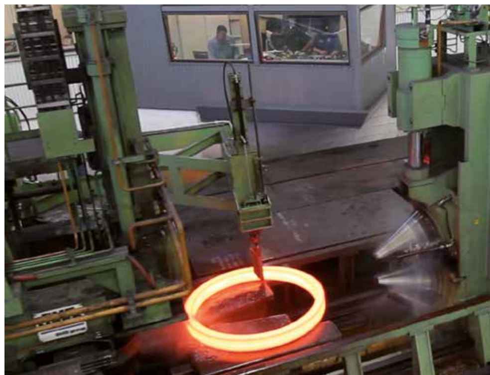
An overhead view of the ring making process.
